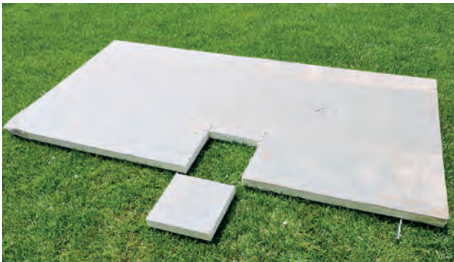
Figure 5. 17 year old polyiso sample
