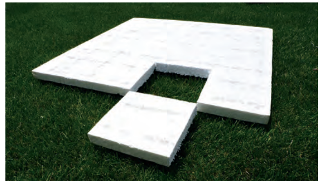
Figure 6. 17 year old Molded polystyrene sample
